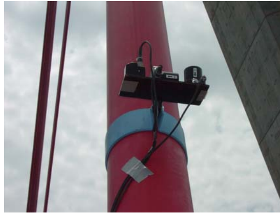
Figure 4.1 Mounting of Sensors at Three Directions
