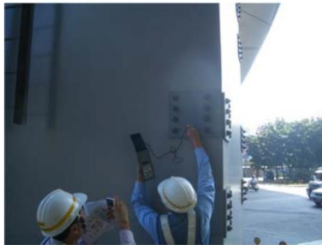
(c)加勁板面漆塗裝模厚檢驗
