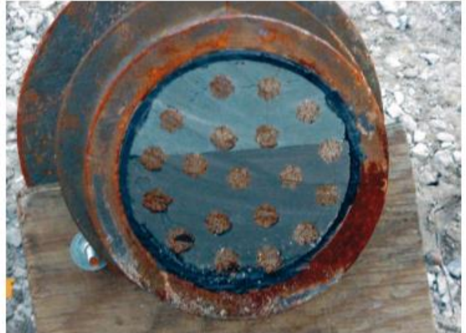
Result of void grouted with Vacuum Grouting
