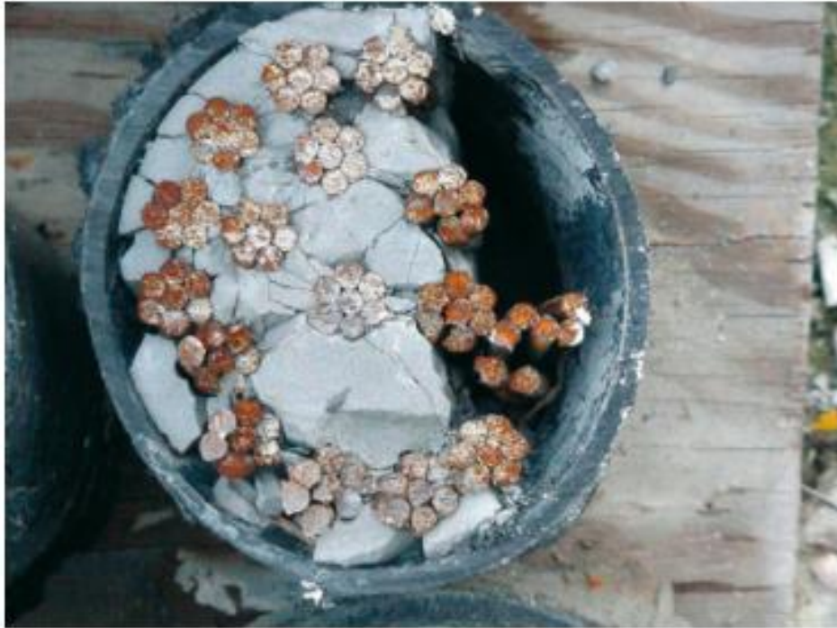
Result of void grouted with conventional methods
