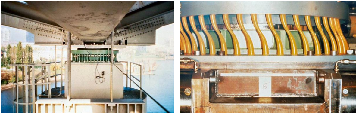
Figure 19: Slider with steel hysteretic dissipating elements installed in the Marquam Bridge, Oregon, USA (left) and the prototype under testing in FIP Industriale's laboratory (right).
