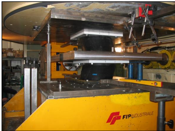
Figure 5: Elastomeric Isolator under testing (right) and typical HDRB hysteresis loop.
