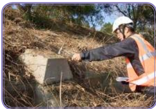
(a) Appearance check on the protection seat
