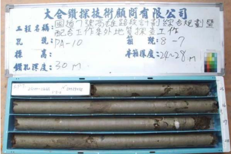
PA-10 鑽孔岩心箱照片(24.0 M ~ 28.0M)
