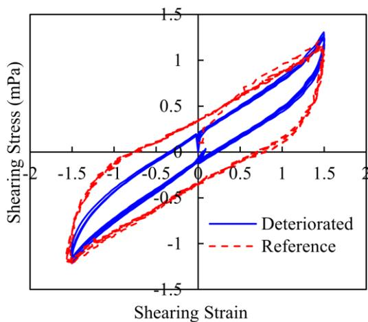
Figure 10. Remaining seismic performance of damaged LRB shown in Figure 9(a) (150% shear deformation test result)
