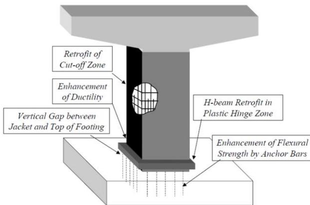
Figure 3. Concept of steel jacketing method with anchor [UNJOH et al, 2008]
