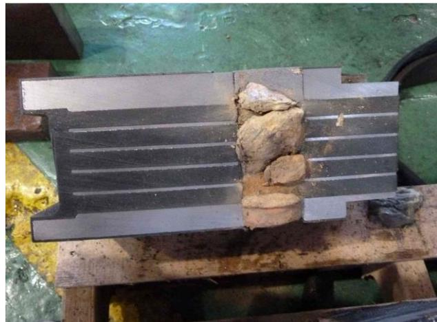
Figure 11. Fragmented lead plug of damaged LRB shown in Figure 9(a)
