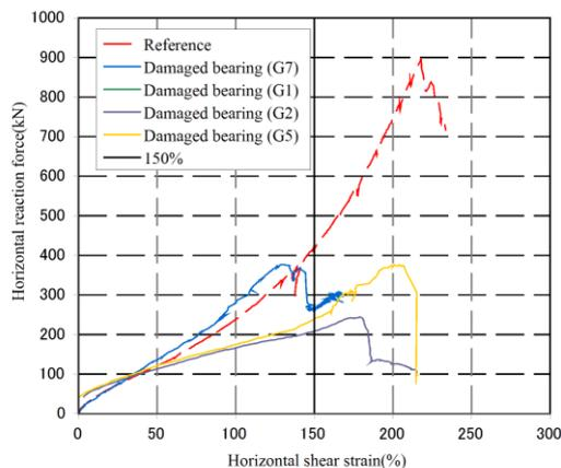
Figure 12. Remaining seismic performance of damaged RB shown in Figure 9(b) (Ultimate shear strain test result)
