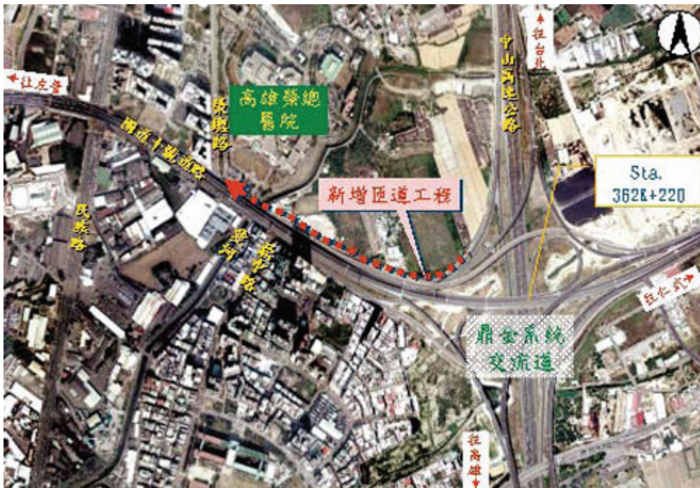
Elevated Ramp Works of Freeway No.1 Dingjin Sytem Interchange Additional Southbound Right Turn Lane Connecting to Freeway No.10
