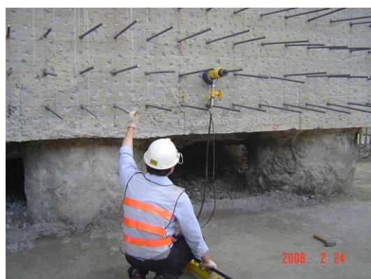
10.植筋拉拔試驗
