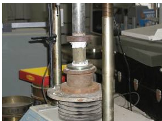
13.試體單壓強度試驗
