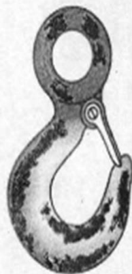
EXCESSIVE RUST OR CORROSION
