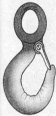
WEAR OR SCRAPING
