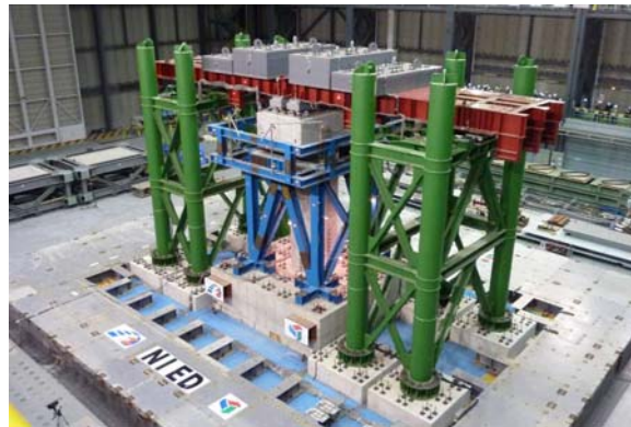
Photo 1. Experiment set-up using E-Defense shake table
