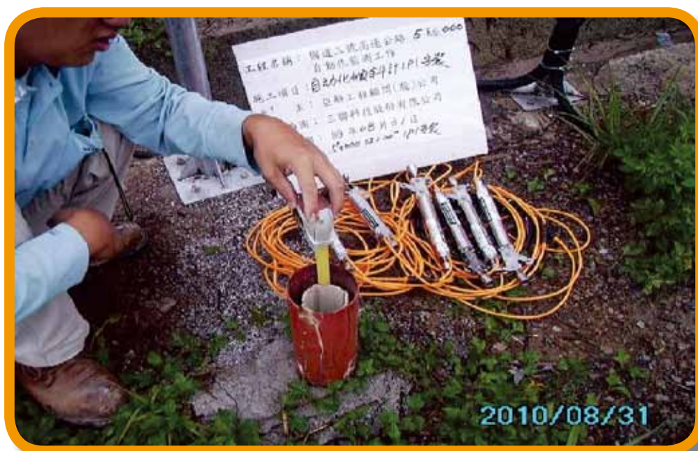
Fig. 2: Automated measurement of tilt tubes
