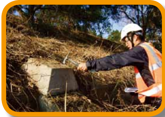
(a) Appearance check on the protection seat
