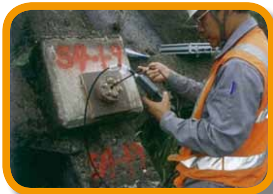
(c) Endoscope inspection
